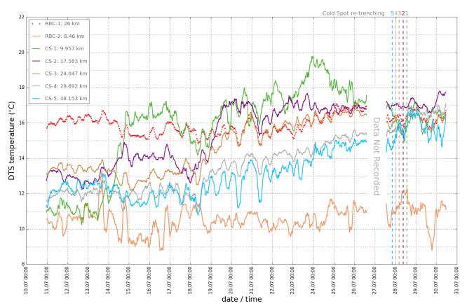
Fig. 5: DTS time series (10-31/07 2018) for Cold Spot positions CS-1 to CS-5 and Reference Buried Cable sections at 8.46 km and 26 km. The timing of the re-trenching operations (starting at CS-5) is also indicated
