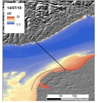
Fig. 6: The 14/07/18 Seabed temperatures from the UK Met Office FOAM AMM15 model. The direction of flow of the warm Jutland Coastal Waters is shown in grey
